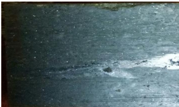
Figure 3: Brake Shoe Surface After Test
